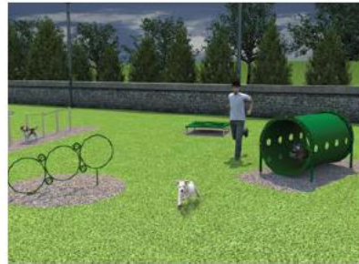
Small Dog Course: For those individuals that own a smaller dog, this features a hoop jump that is closer to the ground and smaller, making it just the right size for teacups and terriers. The suggested minimum use zone is approximately 19' x 23'.
